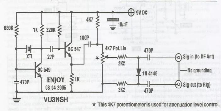
Use high frequency high speed diode for UHF and above frequencies
