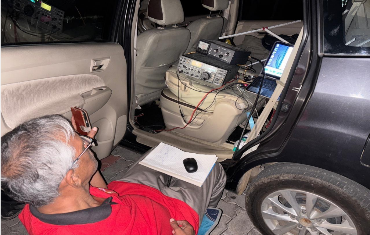
Wg Cdr Sampath, VU2SAA, operating from his mobile shack. HF Rig Icom IC-745 with Comet manual tuner. Inverted V Fan Dipole antenna for 7,14 and 28 MHz. The vhf rig was FT 7800, The antenna was a homemade 3el tape Yagi. The whole station including laptop was operated using power sourced from car battery.
