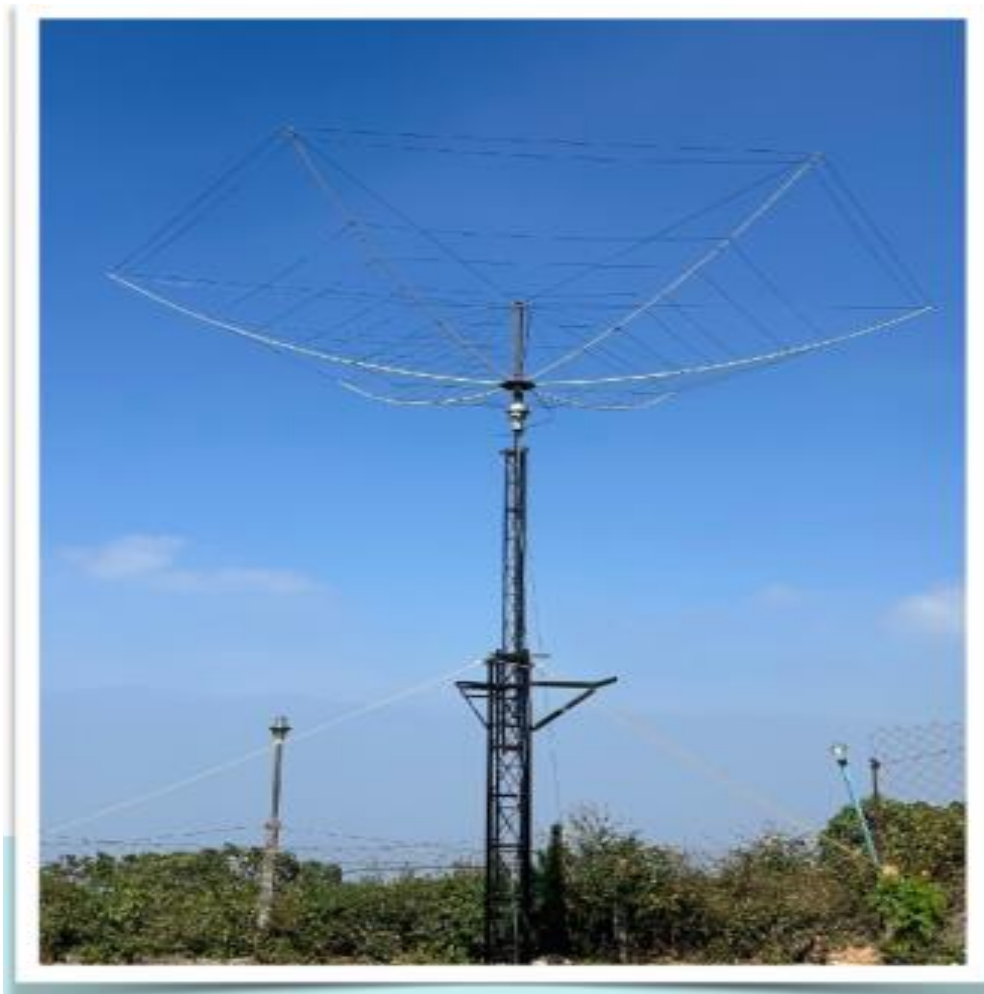
The six-band Hex-beam at AT3N – portable station during ARSI Field Day & Hill Topping contest 2024
