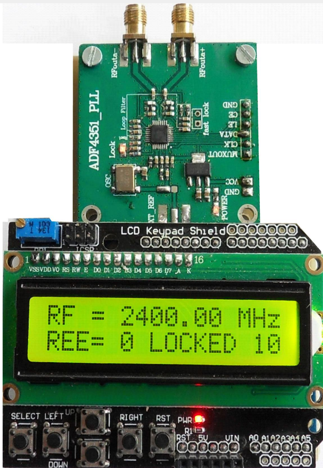
Fig.10 Test Generator module ADF 4351 controlled by Arduino Uno.
