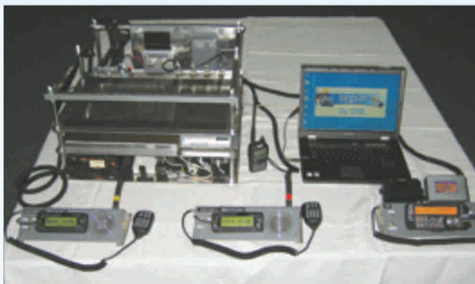
Figure 1 — Three control heads removed from the base are displayed close together, but each can be relocated a distance of 8 feet from the base. The IC-91AD handheld transceiver has been removed from its storage bracket on the lower shelf. The laptop can also be moved the full length of its cabling when using pactor or packet.
