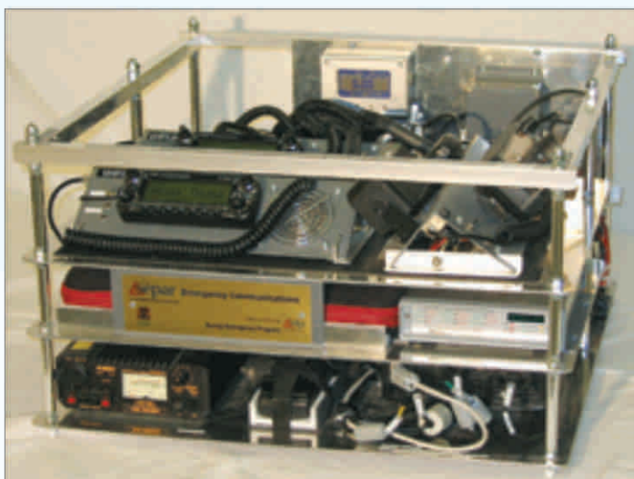
Figure 3 — The radio kit, plus manual pouch and utility case (containing headphones, laptop power cables and CW keyer) all fit snugly inside a Pelican 1640 case.
