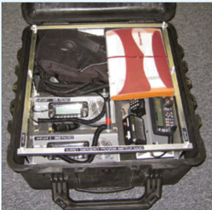
Figure 3 — The radio kit, plus manual pouch and utility case (containing headphones, laptop power cables and CW keyer) all fit snugly inside a Pelican 1640 case.
