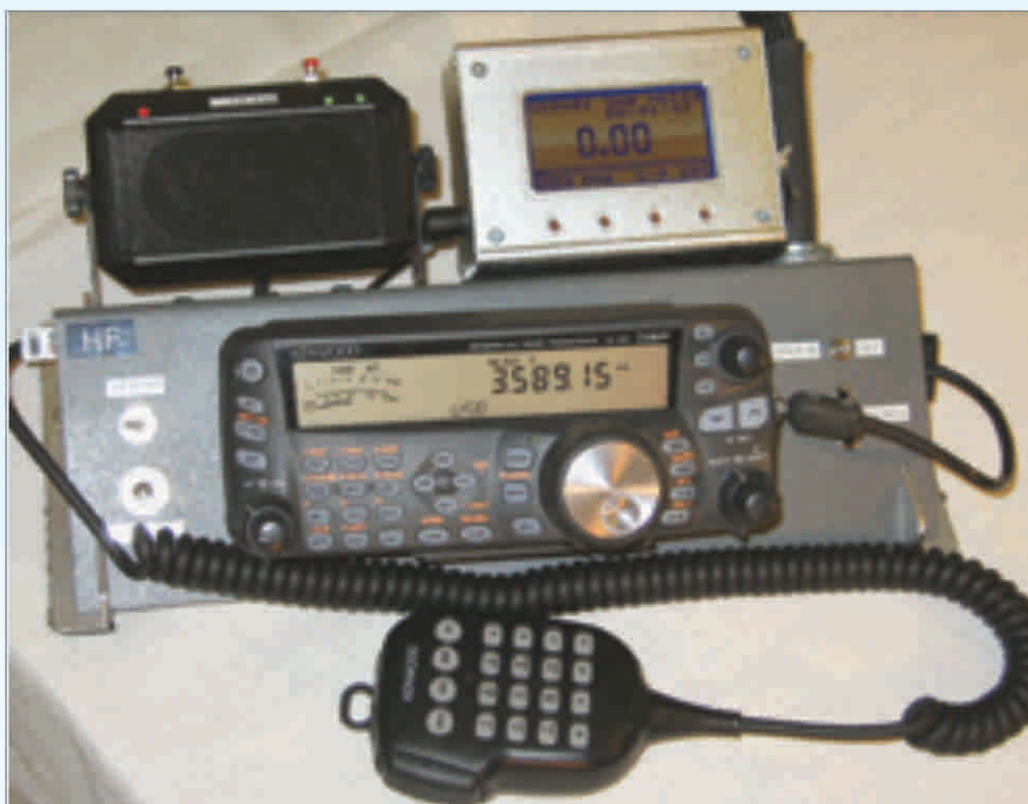
Figure 2—The TS-480SAT control panel with the SGC noise canceling DSP speaker fastened to the back. In this view, the VE7XDT power/SWR meter has been relocated from the base to the control head and is held in place by Velcro—both 12 V and a signal cable must be provided at the control head for the meter to function at this location. When the meter is not in place, the spot is occupied by the hand microphone.
